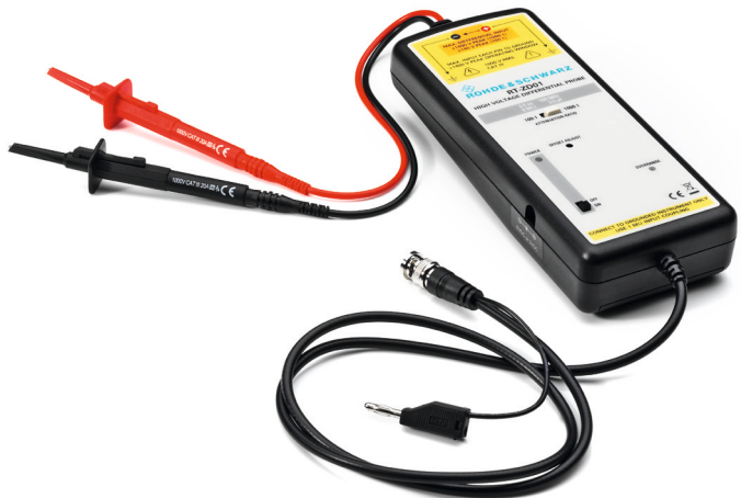
R&S®RT-ZD01 high-voltage differential probe (100 MHz, 1 kV (RMS)).
